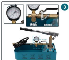
Fig. 3 - Valve closed, pressure check
